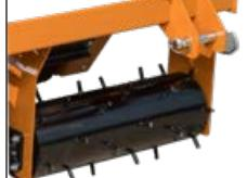
1. Choose a spiked roller with adjustable angles that will penetrate thatch and aerate lawns, or angle it to break up the surface and remove stands of turf.
