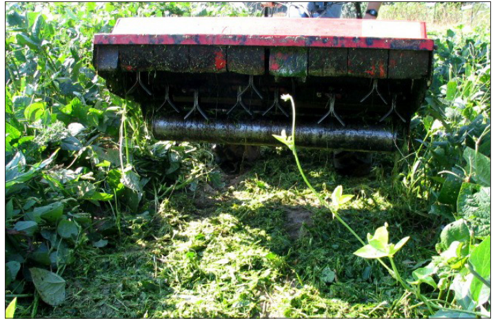
Figure 7. Flail mower used to terminate cover crops.
